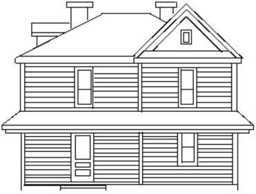
**Appropriate** Siding should be replaced with materials which duplicate the original in size, shape, and texture.
