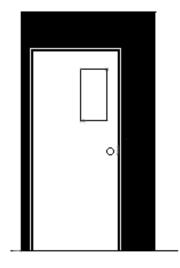
**Inappropriate** The original door has been blocked down.
