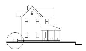
**Inappropriate** Avoid the installation of mechanical equipment on the street façade.
