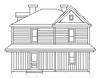
Inappropriate Siding should be applied horizontally.
