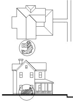
**Appropriate** Mechanical equipment installed on the street façade should be screened from view.
